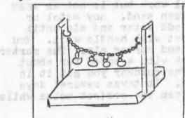
A BRACTLET STAND is another simple aid easily made from 3 pieces of wood and 2 cup hooks. This will be helpful in assembling bracelets and in counting off links for accurate separation of stones.
