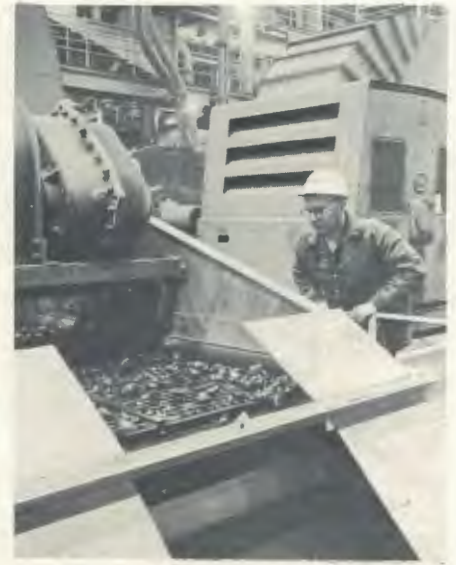
The iron in the crude ore (now much finer than face powder) is recovered by these magnetic separators and pumped as a pulp to . . .
