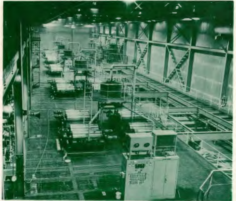
The iron in the crude ore (now much finer than face powder) is recovered by these magnetic separators and pumped as a pulp to . . .
